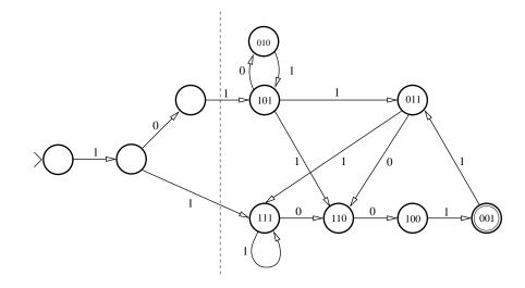
Figure 10: The automaton recognizing the language  $\mathcal{L}_Y$  of Example 3.4.
